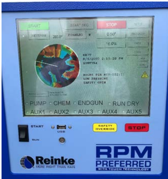
Picture of control panel showing the irrigation pattern
