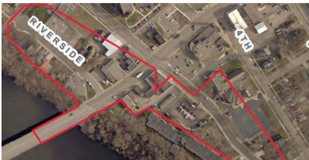
Drainage area the 2020 sump structures will treat
